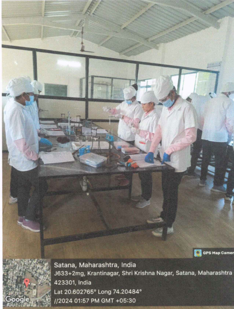
Proper PPE kit for handling of Hazardous chemicals and waste
